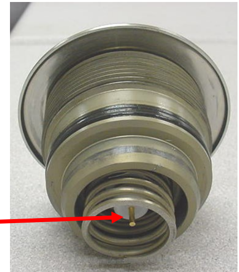
COAXIAL CABLE FROM THE INDICATOR TO THE HOUSING
